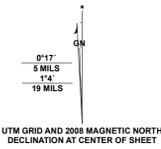
UTM GRID AND 2008 MAGNETIC NORTH DECLINATION AT CENTER OF SHEET
